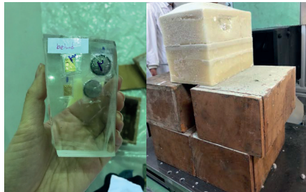
Figure 7: Neutron transmission measurement of sapphire with 5.5 cm thickness, right: experiment setup in front of radiography channel of TRR.
